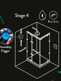
User switches shower off, Humidity Trigger passes information to Nerve Centre and the fan airflow is reduced automatically to 8 l/s.
