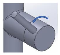
To operate the Filtered water on the 4-in-1 Tap, pull the H/C handle forward.
