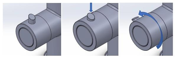
To operate this handle, it requires a firm force being pushed down on the spring-based button followed by a first twist away from the front, pushing all the way to activate the Boiler feed water.
