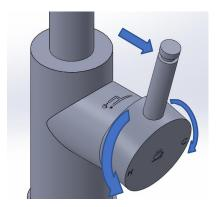
To operate this single lever, first push out the handle and pull either forward or backwards as shown by the indicator on the body.
