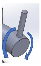
Pull the lever away from the body of the tap for mixed H/C water. Rotate Towards the indicated H for Hot water or C for Cold water to adjust the mixing of the tap.
