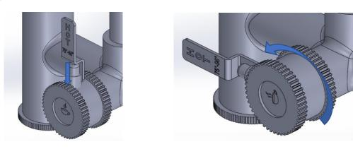
For this Handle first press the HOT tab downward, then rotate the handle left to activate the Boiler feed water.
