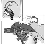
Make sure the float moves freely after this adjustment has been carried out, or the inlet valve will not shut off or will be in shut off position.
