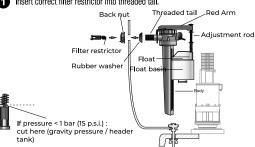
2 Fit the filling valve. Ensure that the valve does not obstruct the flush mechanism. Do not overtighten the back nut.
