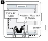
Install a 50 mm deep electrical back box in your preferred thermostat location. Pull wires (heater, supply and sensor(s) through back box and complete terminal wiring.
