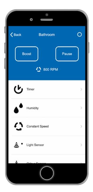
7. Select the **E** Timer function in the Function menu to customise the Fan Speed on this setting between 800 and 2400 RPM, the Running Time and the Delay Start settings.
