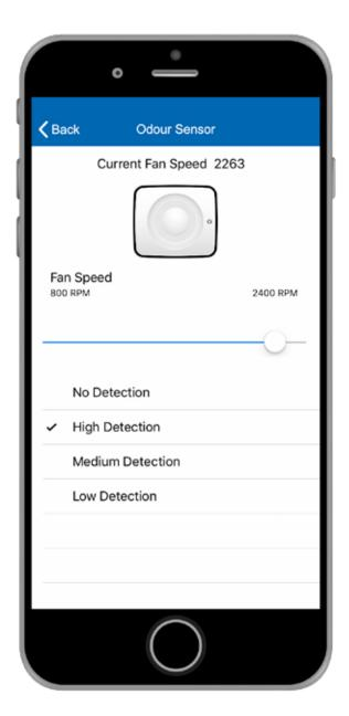
12. Select the Airing function in the Function menu to customise the Fan Speed on this setting between 800 and 2400 RPM.
