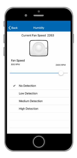
9. Select the Constant Speed function in the Function menu to customise the Fan Speed on this setting between 800 and 2400 RPM.
