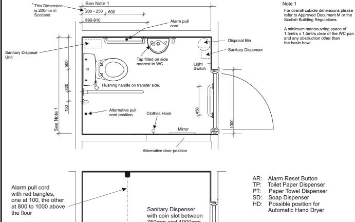
Sanitary Dispenser with coin slot between 750mm and 1000mm above the floor
