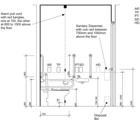
The drawing above shows a Left Hand installation. A Right Hand installation is the mirror image of above.
