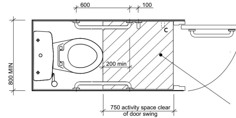
The area shown is the minimum required. It must be clear of all obstructions (eg plumbing and drainage fittings).
