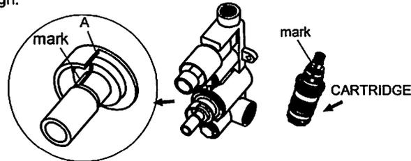
4. Fit the stop lug and handle body with part A and B (fix stopper) aligned. Then screw and tighten handle lever.
