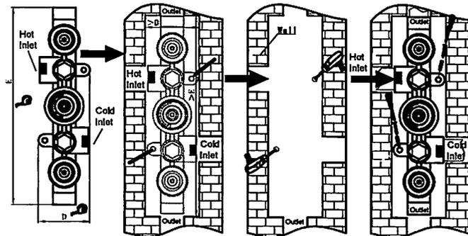
2. Marked secure the concealing plate onto the valve body which is clearly marked. Then fit the rubber washer, handle body, grub screw and hand lever.
