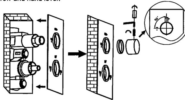
3. Factory outlet setting temperature is 38°C when face A aligns the align mark on the cartridge. Do not turn the spindle in case of any movement, which will result in an incorrect factory outlet temperature 38°C. If this is the case, please as shown below re-align.
