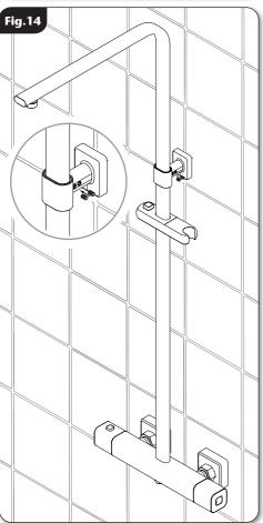
Secure the rail to the bracket with the supplied grub screws **(fig.14)**.
