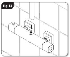
Push the assembled rail onto the valve, taking care not to damage the O-rings (fig.13).
