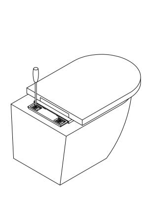
WITH THE FIXING PLATE AND BOLT SETS IN POSITION, SLIDE THE PLATE BACK INTO THE HINGE PLATE 5mm ONLY AS THIS WILL ALLOW ACCESS FOR TIGHTENING THE BOLTS.
