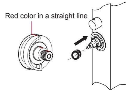
④ Press the button on the valve and put on the head as below ensuring the screw hole pointing to the front
