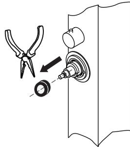
⑤ Unscrew the brass ring from the valve using the tool
