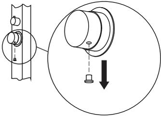
② Loosen HEX screw off with hexagonal wrench
