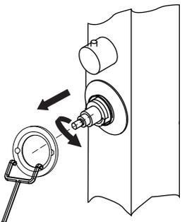
⑥ Remove the valve and clean: Run under warm water and use a toothbrush or similar to remove any debris or limescale
