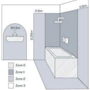
Suitable for indoor only. This product is rated as IP24. If the product is to be installed within a bathroom it can only be located within zone 3.
