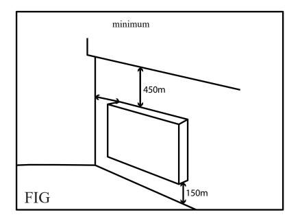
Please use the mounting brackets supplied. The heater should be positioned observing the minimum clearances stated around the heater – see Fig. 1
