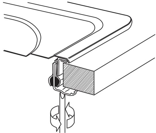
Do not overtighten the fixing clamps once the sink is fully bedded in the sealing tape. Do not tighten fully at the first attempt.
