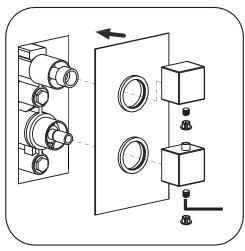
Once the mixer has been fitted and secured, push the concealing plate over the mixer body, sealant should be applied between the plate and the wall.
