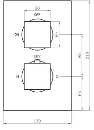
Your product is factory set under balanced pressures, with specific inlet temperatures, as your site conditions may differ, the temperature stop position may require re-setting, to achieve the 38 °C.
