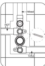
Offer the mixer into the recess and mark fixing locations.
