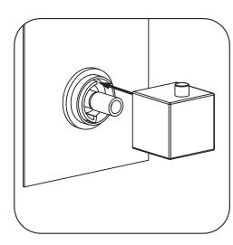
Fit temperature control handle to thermostat, ensuring the stop pin inside the handle, is located against the top of the stop ring.
