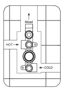
Prepare pipes in wall to connect to shower, with cold on the right.
