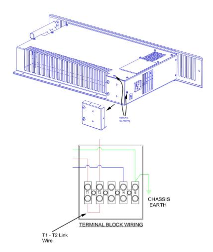
2. Remove T1 – T2 link wire (See above diagram) and connect room thermostat (not supplied) following the manufacturer's instructions.
