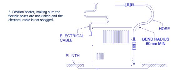
6. Fix the heater to plinth using fixing screw holes located at either end of grille.
