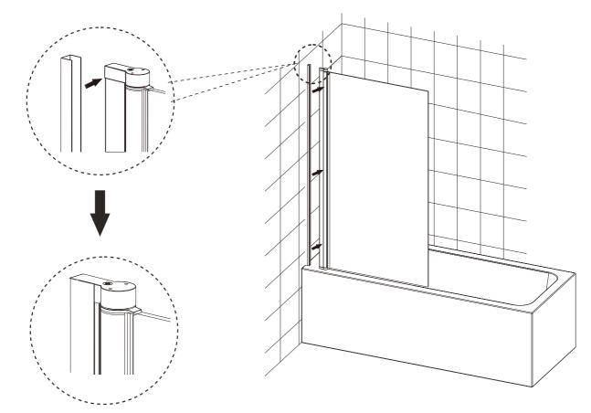
NOTE: To ensure the screen is parallel to the bath hold the top of the hinge and move the whole screen back or forwards to adjust before carrying out step 3.
