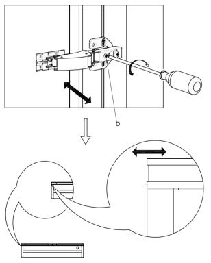
Rotate CW: Door moves to the center of the mirror cabinet Rotate CCW: Door moves to both sides of the mirror cabinet
