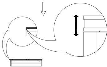
Rotate CW: Distance between door and cabinet reduces Rotate CCW: Distance between door and cabinet increases
