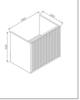
Dimensions (measurements in mm)
