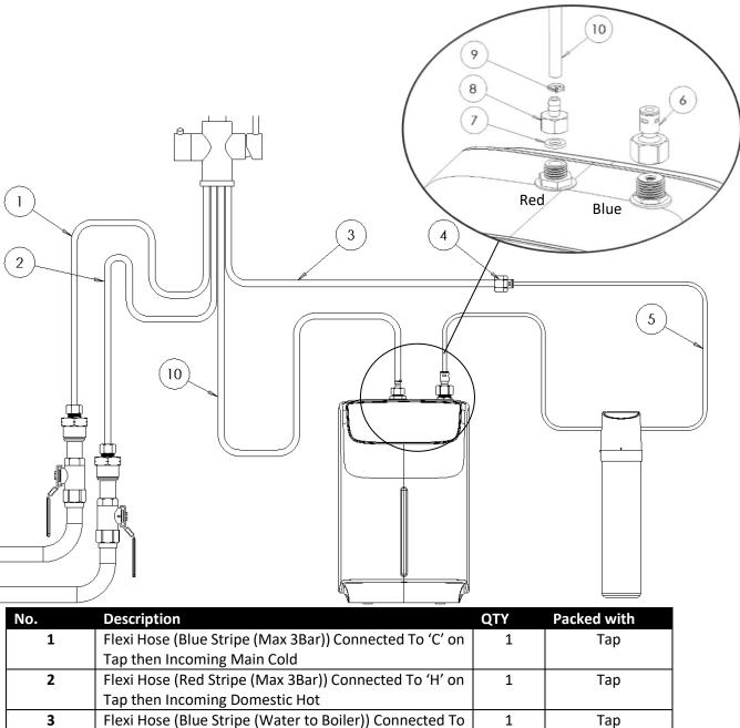
For servicing purposes, the services provided by the customer should have means of isolation. These should terminate with  $\frac{1}{2}$ " BSP male fittings to accept the tap flexible tails (1 and 2).
