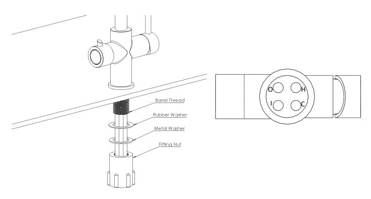
Feed the tails through the barrel thread and hand tighten into the tap. Fit the tap in the desired location using the black plastic fitting nut.
