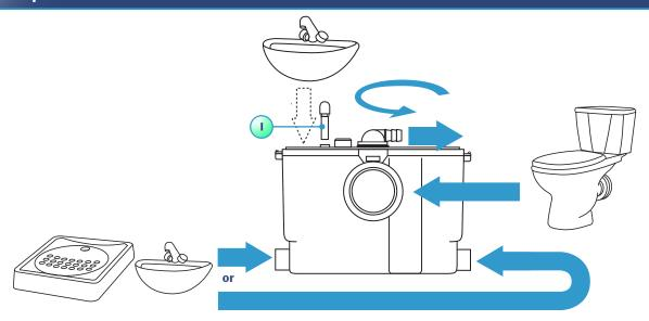
This unit is a compact pump/macerator specially designed to take the waste from a wall hung or back to wall WC pan. It will pump away the waste from one WC, one washbasin, one shower and one bidet.
