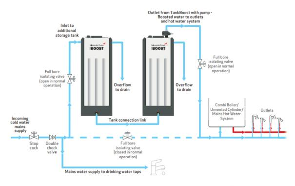
Additional storage tanks must be the same capacity as the main TankBoost unit.
