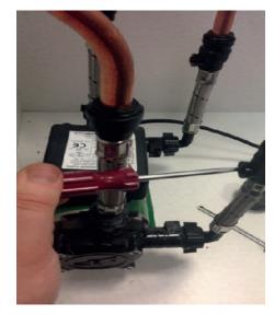
Both sets of hoses can now be removed from the pump - there will be some residual water in the hoses and pump, so it may be worth using a cloth to catch the excess.
