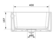
NB: Due to manufacturing processes this sink may have a +/- 5mm tolerance on the measurements.
