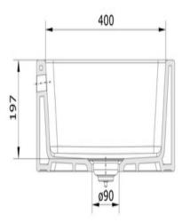
NB: Due to manufacturing processes this sink may have a +/- 5mm tolerance on the measurements.
