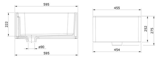
NB: Due to manufacturing processes this sink may have a +/- 5mm tolerance on the measurements.
