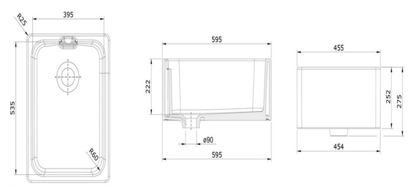
NB: Due to manufacturing processes this sink may have a +/- 5mm tolerance on the measurements.
