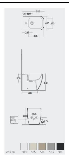
Dimensions: All dimensions in mm. Tolerance of vitreous china & fireclay items: ± 5% for below 200mm and ± 3% for above 200mm; for all other items tolerance ± 1%. Note: Due to a continuing development program to improve design and performance, the manufacturer reserves all rights to vary specifications without prior information. Please note accessories are for photographic use only.
