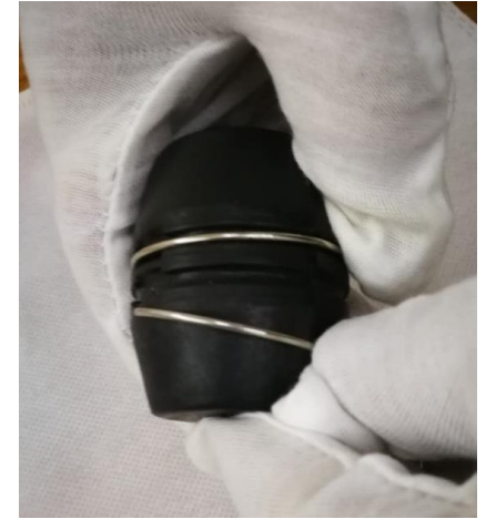
Step 5: Take off the rings from the Weight by hand
