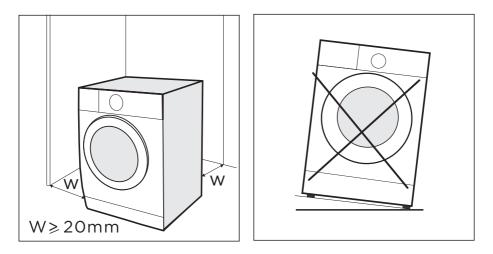
Before installing the machine, the location characterized as follows shall be selected: 1. Rigid, dry, and level surface.
