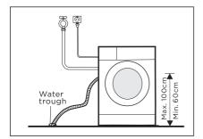
2.Connect it to the branch drain pipe of the trough.
