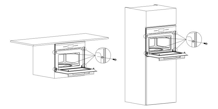
Note: Do not take the door handle as force bearing point during the installation and removal.
