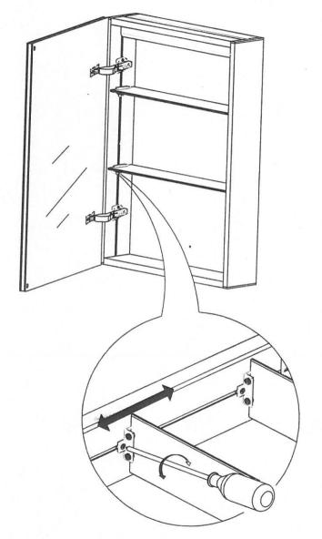
Loosen the screws can adjust the distance of the glass shelves
