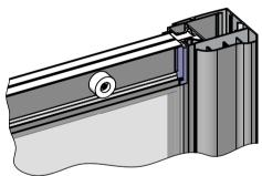
IF THE ENCLOSURE OR SIDE PANEL HAS THE OPTIONAL SCREW COVER PROFILES (ITEM 2) PUSH FIT THEM ONTO THE SCREW COVER PROFILE
