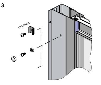
WHEN THE ENCLOSURE IS READY TO BE FIXED, DRILL THROUGH THE HOLES IN THE WALL PROFILE AND CORNER POST WITH A 3mm DRILL. (MAKE SURE YOU ONLY DRILL THROUGH ONE WALL THICKNESS) THEN FIX THE FRAME WITH ITEMS 10, 11\* & 12\*.
