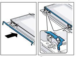
12. Attach the door cover 1 and use a screw to secure it on the left- and right-hand sides ②.
