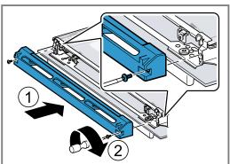
Slide the appliance door straight onto the two hinges. Slide the appliance door on as far as it will go.
