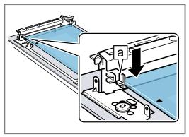
**4.** Slide in a second intermediate pane. When doing so, ensure that the number on the intermediate pane is at the bottom right ①.
