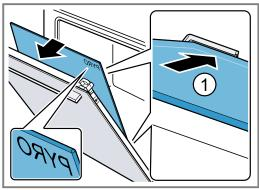
**5.** Push the inner panel in at the top ①. Push the sliding caps a downwards in the direction of the arrow.
