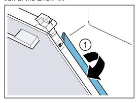
8. Pull the first and second intermediate panes upwards and out at an angle, and set them down carefully on a flat surface.
