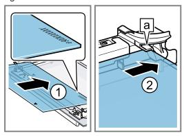
6. Push the intermediate pane upwards until it is in the retainer a.
