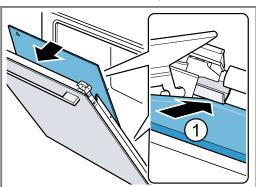
2. Note: The intermediate panel is automatically positioned by the rotational movement of the spacer.
