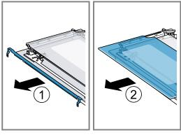
**9.** Loosen the screw on the left- and right-hand spacers a ① and remove both spacers ②.
