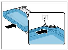
10. Push the inner pane upwards until it is in the leftand right-hand retainers a.
