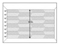
**7.** Install the remaining material, in alternating rows of "A" and "B" planks. Drop and lock the end joints together and keep square throughout the install.
