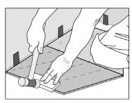
Pay close attention when lining up the chevron pattern alignment (point to point). Make sure there are no gaps and the points line up per-fectly. Tap along the long-groove edge using a profiled tapping block and soft-faced hammer to ensure the joint is closed fully (Figure 4B). NOTE: Always square long side joints BEFORE tapping down short joints.
