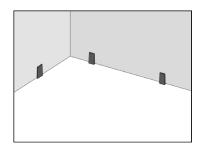
1. Create the required expansion space between the perimeter planks and the wall using spacers. Place spacers equaling the thickness of the required ex-pansion between plank and wall on short and long ends of plank. Do not remove the spacers until the installation is complete.
