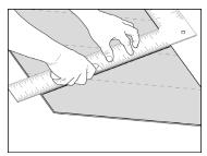
**6.** Install the last two pieces of rows 1 and 2 by cutting to fit. Maintain the expansion gap and install as before.
