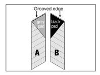
**3.** There are "A" Planks (with a pre-attached grey padding) and "B" planks (with a pre-attached black padding). Separate the A and B planks from the carton. Continually blend the planks from 3 to 4 cartons at one time to ensure a mix of pattern and shade.
