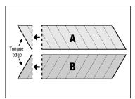
**4.** Starting in the left corner of the room, take a full "A" and "B" plank and remove the angle from the tongue edge of both planks (Figure 4A). Position the "A" plank with long tongue edge against the spacers previously placed along the starting wall (Figure 4B). Interlock plank "B" by inserting the tongue into the groove of plank "A".
