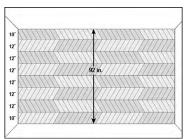
**2.** Identify the direction the chevron planks are to be installed lengthwise. Divide the width of the room by the width of one plank (302 mm). This gives you the number of rows of planks. If one row is less than a full plank (302 mm), you may need to trim the first and last row to balance out the room.
