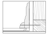
**9.** Remove spacers. Cover expansion space with quarter round or other trim, being sure not to trap or pin down the floor.
