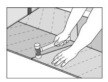
**5.** Create the required expansion by placing 3/8" (10mm) spacers between the flooring assembly and the walls. Do not remove the spacers until the installation is complete
