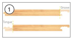
Hydrolock panels are supplied as standard with a tongued long edge and a grooved long edge. When fitting panels into an extrusion, the protruding tongued or grooved edge should be cut off.
