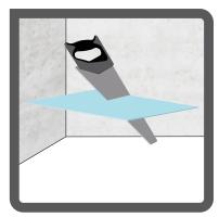
When using a fine-tooth blade handsaw, panels should be cut decorative face up.
