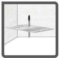
When using an upward cutting blade (jigsaw) or a circular saw, panels should be cut face down to avoid chipping.
