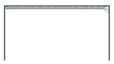
Push panel into internal corner and press against wall firmly, clean any excess silicone from corner.
