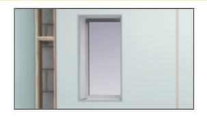
At windowsills, a Type E quadrant end cap should be used between panels, and mitred in the corners.
