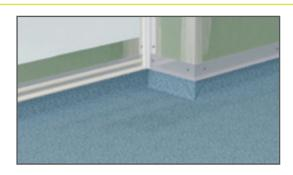
In wet areas, such as wetrooms, we recommend the use of an aluminium Type X base profile. Height adjustments should be made where the panel meets the ceiling. Floor covering material should continue approx. 100mm up the wall behind the panels. Screw fix the profile through the floor covering into the wall/frame, and apply silicone sealant to the base and the back of the profile.
