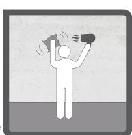
To ensure your Multipanel® is properly bonded, ensure all surfaces to which adhesive will be applied are clean and dry.
