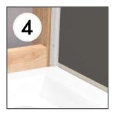
The first profile, which normally starts with an Internal Corner or End Cap, should be fixed to the wall or end grounds with countersunk screws, or adhesive and a bead of silicone sealant applied to the channel.
