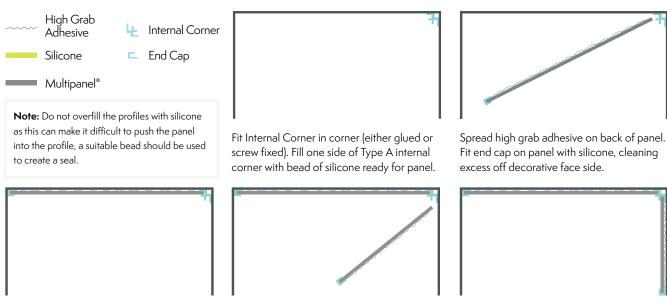
Push panel into internal corner and press against wall firmly, clean any excess silicone from corner.
