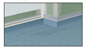
In wet areas, such as wetrooms, we recommend the use of an aluminium Type X base profile. Height adjustments should be made where the panel meets the ceiling. Floor covering material should continue approx. 100mm up the wall behind the panels. Screw fix the profile through the floor covering into the wall/frame, and apply silicone sealant to the base and the back of the profile.
