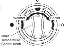
**3.** Turn the outer flow control knob fully **clockwise** to stop the flow of water.
