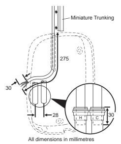
Make sure that the end of the supply pipework is cut squarely and is free from burrs, which will damage the inlet manifold seals.
