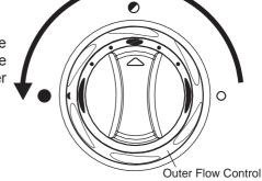
2. Turn the inner temperature control knob anticlockwise for warmer water and clockwise for cooler water.
