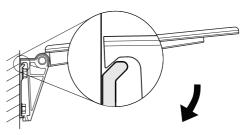
8. Secure the shower seat to the wallplate with the grubscrew. Make sure that the seat pivots up and down freely.
