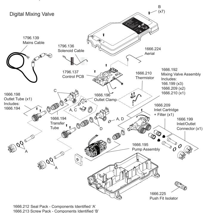
1666.197 Solenoid - Components Identified 'C'
