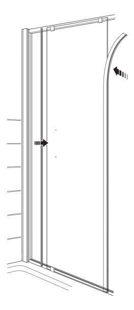
(a) Install the seal to one side of the door and the magnetic door seal to the closing side, ensuring that the magnet attracts to the wall channel.
