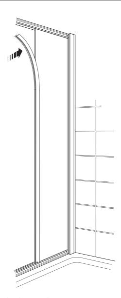
(a) Install the seal to the glass panel.
