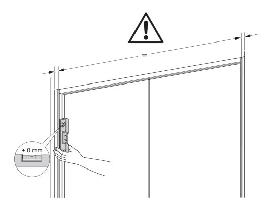
(a) Centralise the door frame within the wall channels, making sure that the door frame is square.
