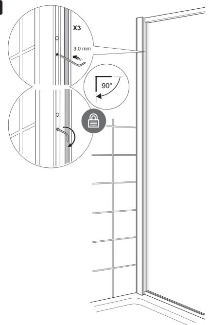
(a) Using the 3.0 mm hexagonal wrench (supplied), turn through 90° clockwise to lock the door frame in position.
