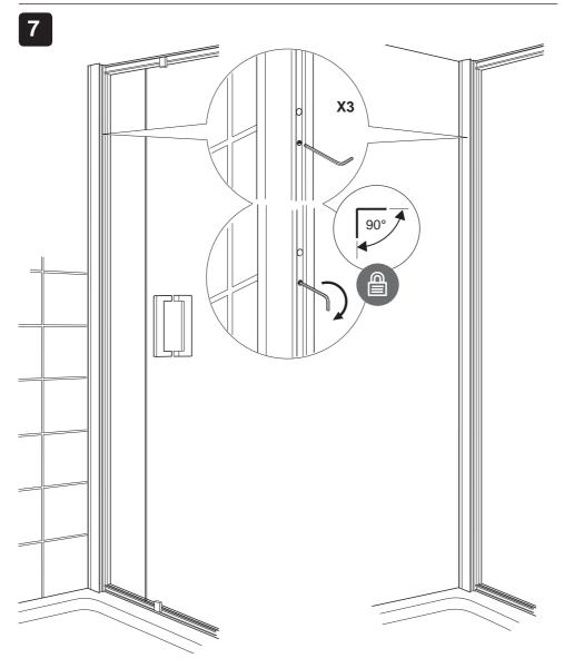
(a) Using the 3.0 mm hexagonal wrench (supplied), turn through 90° clockwise to lock the door frame, corner post and side panel in position.
