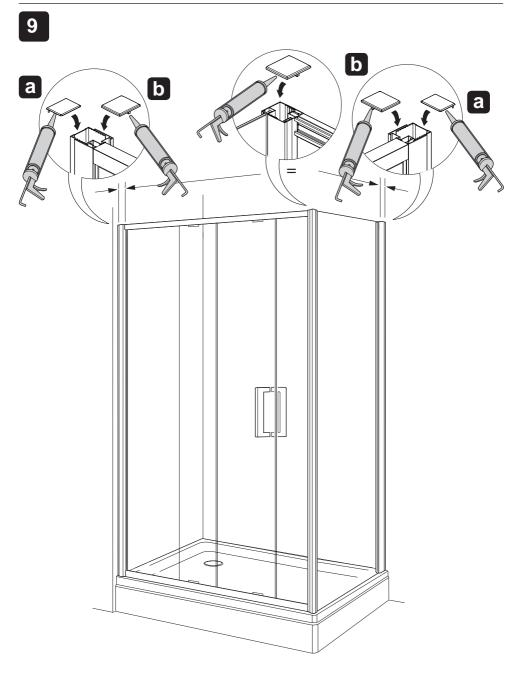
(a) Fit the plastic covers to the top of the extrusions.
