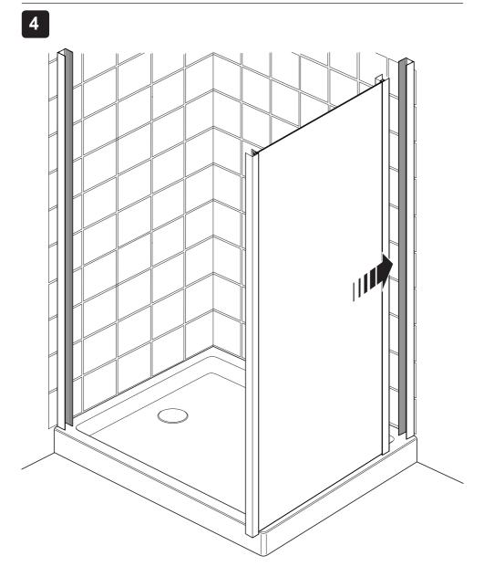
(a) Install the side panel into the wall channel and hold in position.
