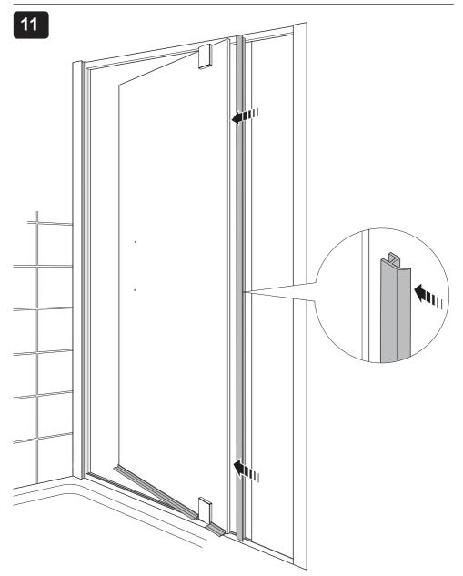
(a) Install the panel seal to the door shown above.
