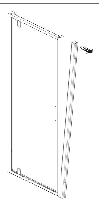
(a) Remove the wall channel.from the door.
