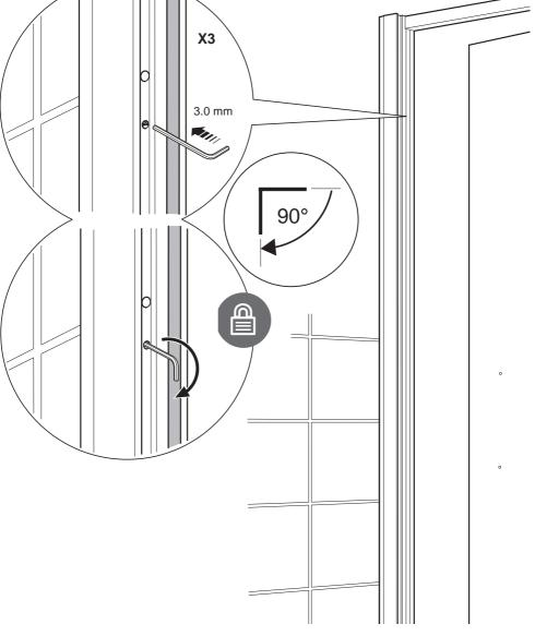
Using the 3.0 mm hexagonal wrench (supplied), turn through 90° clockwise in (a) three locations to lock the door frame in position. Repeat this on the other wall channel.
