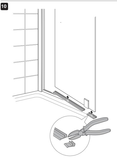
(a) Install the splash seal to the door as shown above.
