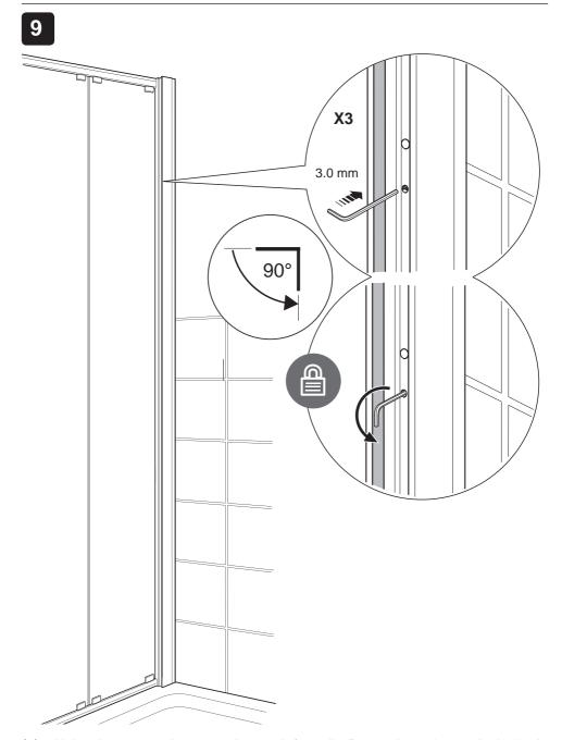
(a) Using the 3.0 mm hexagonal wrench (supplied), turn through 90° clockwise in three locations to lock the door frame in position.
