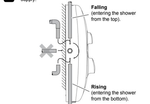
**Note!** - **DO NOT** use an incoming supply entering the shower directly from the back. Add an elbow to the supply pipe and connect it as a rising or falling supply.
