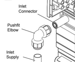
Connect the inlet supply pipe to the inlet connector using a push fit elbow or an elbow with compression nuts and olives.
