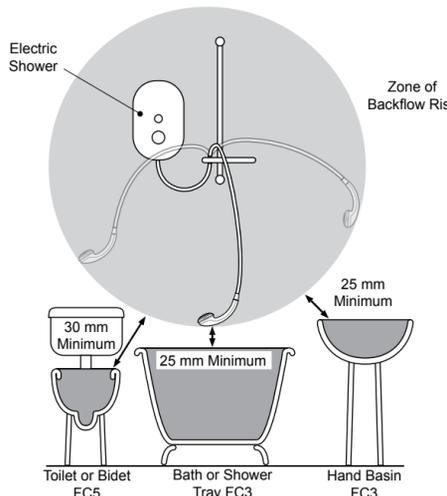
**Hose retaining ring fitted and shower fittings fixed at a suitable height preventing dirty water backflow.**
