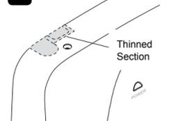
For falling or rising supplies the cover has thinned sections on the top and bottom that can be removed to allow entry of the supply pipe and electrical cables.
