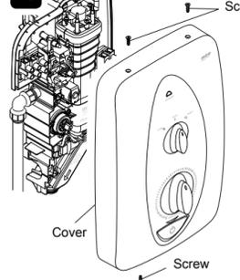
Ensure the control dials are aligned with the spindles and replace the cover.
