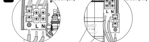
Terminal Blocks are provided on both the left and right for convenience. Use the terminal block location that is most appropriate for your installation i.e. If the electric supply is on the right hand side then use the right hand terminal block.
