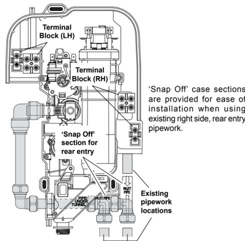
'Snap Off' case sections are provided for ease of installation when using existing right side, rear entry pipework.
