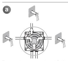
Turn on the water supply and flush the outlets.
