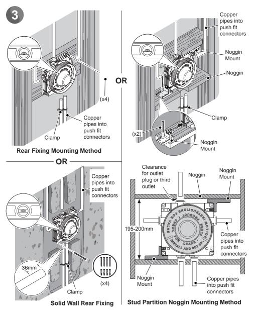
Plan fixing method for product in wall cavity.
