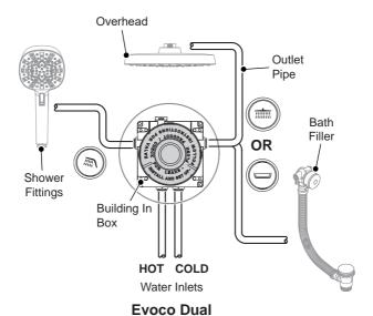
Fit the outlet pipework ready for connection to either a right angle connector for a handset, bath (adjustable fitting), or a shower arm for a fixed spray head (rigid fitting).
