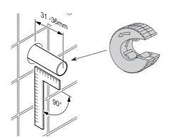
The right angle connector must be fitted to a waterproof, flat and even wall surface.
