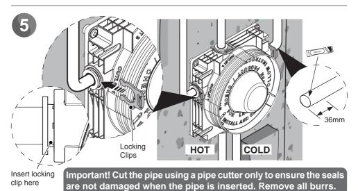
Note: Grease sachets are supplied and a small amount should be applied to the end of the pipe to aid insertion.
