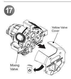
Remove the cover from mixing valve.
