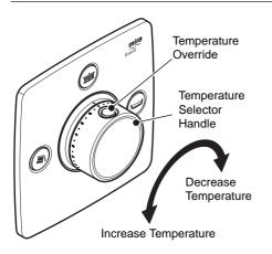
The temperature is controlled by rotating the temperature handle.
