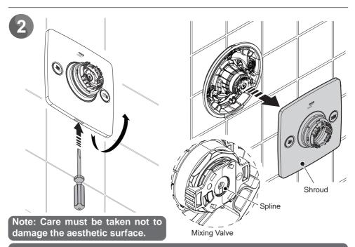
Note: Make sure that the spline is oriented in line as shown above.
