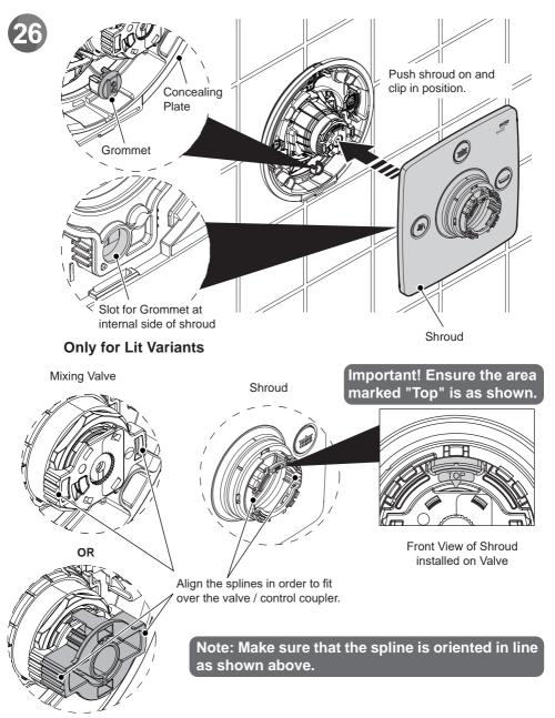
Place the shroud over the valve ensuring the logo is in the correct orientation as shown.
