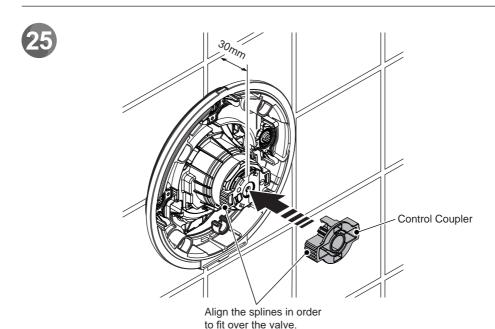
Note: Fix the control coupler if the front of the mixing valve is less than 30mm from tile.
