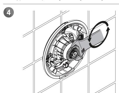
Carefully loosen the hexagonal head nut as shown.
