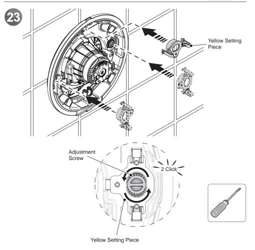
The adjustment screws have to be set to ensure when the concealing plate is fitted the on/off buttons work correctly to turn the shower on and off.
