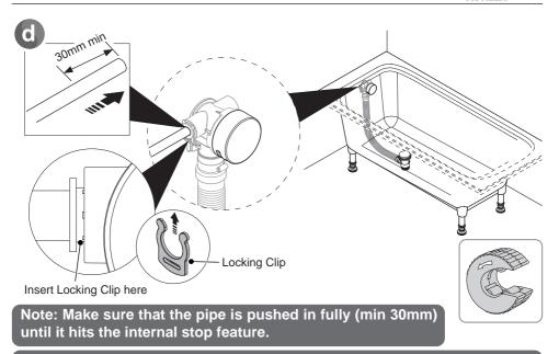
Important! Cut the pipe using a pipe cutter only to ensure the seals are not damaged when the pipe is inserted. Remove all burrs.
