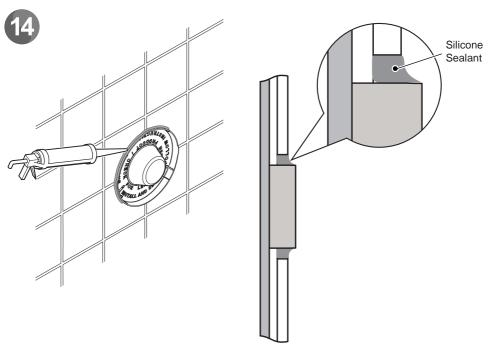
Apply silicone sealant to fill the gap around the Building in Box.
