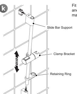
Fit all the components onto the slide bar and fit the slide bar assembly in position, making sure that it locates correctly.
