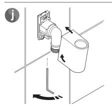
Fit the cover over the elbow and lock into place by turning the grub screw anticlockwise.
