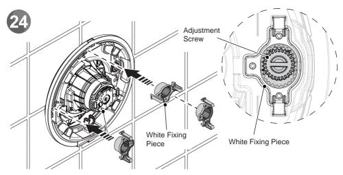
Place the fixing piece over the adjustment screw (as shown). Push and clip the fixing piece to lock adjustment screw in position.
