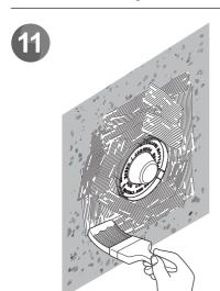
Apply further adhesive over the fabric wall seal and around the sides of the Building in Box.
