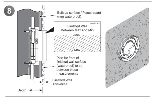
Note: Refer to details of cavity depth and finished wall thickness.
