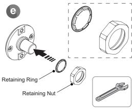
Place the retaining ring and nut over the pipe in the orientation shown and tighten in place using suitable size wrench. **DO NOT** overtighten.
