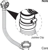
**Note:** When the bath filler waste is extended, there may be a need to rotate the bodies to allow alignment to the both mating surface.
