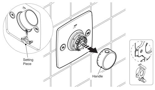
**5.** Remove the maximum temperature peg from the top of the valve by using a screwdriver. Refit the handle.
