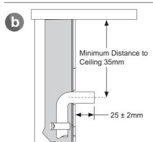
The outlet pipe must protrude 25mm (± 2mm) from the finished wall surface.
