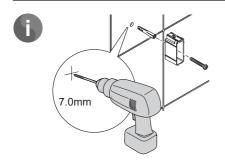
Drill the fixing hole for the top support and fit the wall plug and screw top support into position.
