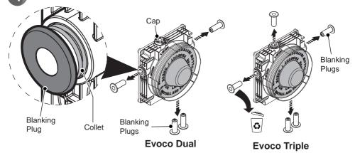
Push and hold the collet before removing the blanking plugs.
