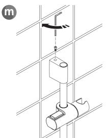
Secure the assembly in position with the screws. The top securing screw tightens Clockwise, the bottom one Anti-clockwise. Do not overtighten!
