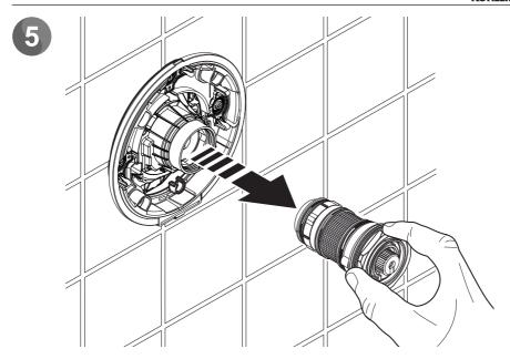
Carefully pull out the cartridge from the mixing valve.
