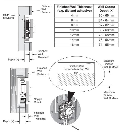
Create a suitable cavity for the Building In Box and the pipework. Cut away the plasterboard and/or brick work to the required depth.
