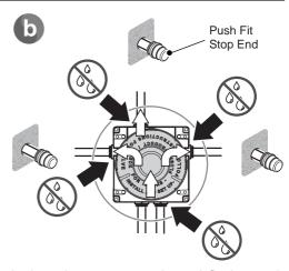
Isolate the water supply and fit the push fit stop ends (not supplied) to the outlets. Re-open the water supply and check for leaks.
