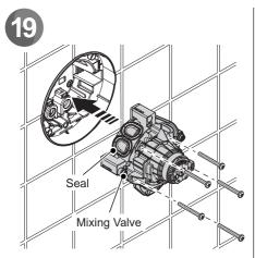
Push in and fully secure the mixing valve into the Building in Box using the provided screws that were removed on step 16. **DO NOT** use a power driver.
