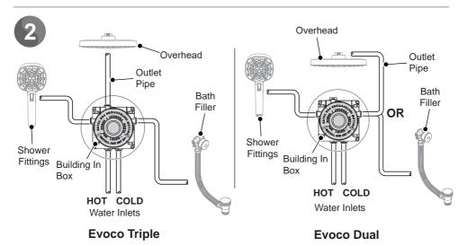
Determine the pipework route. All pipework to the product must be clipped and supported to prevent movement and pipe noise due to any pulse pressures.
