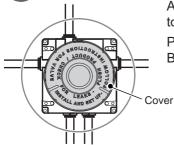
A flushing cartridge is prefitted into the Building in Box to aid in flushing any dirt or debris from the pipework.
