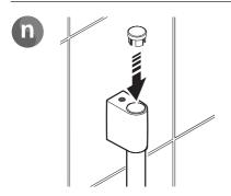
Fit the cap to the top of the slide bar.
