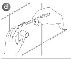
Mark the positions for the fixing holes for the RAC back plate.
