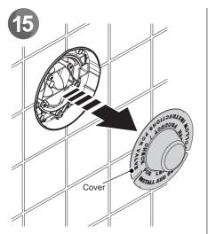
Remove the cover but do not throw away as it can still be used to stop debris during finishing of the installation.
