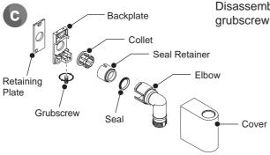
Disassemble the components by turning grubscrew clockwise.
