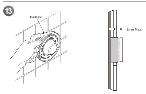
Taking care to prevent damage to the wall finish, trim the Building in Box back to within 2 mm from the finished wall surface.
