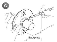
Mark the positions of the backplate fixing holes.
