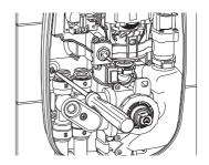
4.7. Using the push-fit release tool, push back and hold the collets from the supply pipework, lift the Mira Event XS T from the wall to remove the supply pipework from the inlet manifold.
