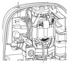
Ensure the green earth wire is connected to the motor.
