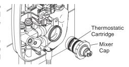
5.5. Fit the replacement thermostatic cartridge. The cartridge must be fitted with the larger lug aligned with the left hand slot in the mixer body and the smaller lug aligned with the right-hand slot.
