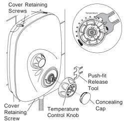
**5.4.** Unscrew the mixer cap and pull to remove both the mixer cap and thermostatic cartridge from the mixer body.
