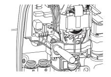
4.6. Remove the three wall fixing screws.
