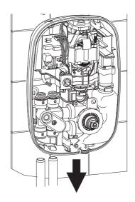
**Important!** This Mira Event XS T **must** be fixed to the wall at all three fixing positions. The fixing holes are elongated to assist in vertical and horizontal alignment.
