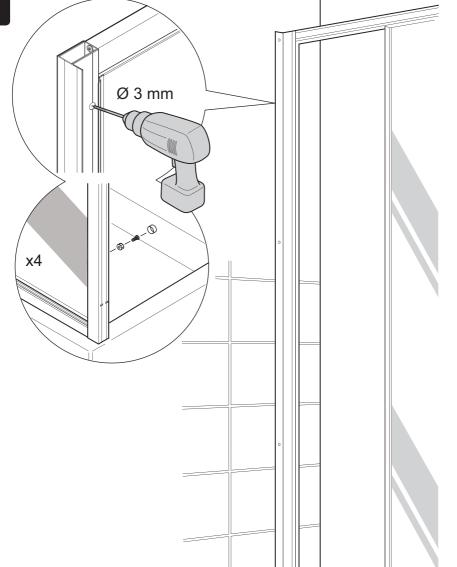
(a) Drill four 3 mm holes from inside the shower enclosure in the door frame through the hole centre marked on the wall channel with a 3 mm HSS drill (not supplied).
