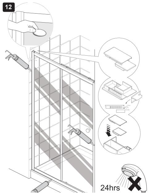
(a) Apply sealant in accordance with the sealant manufacturers instructions along the outside surfaces of the door frame only.
