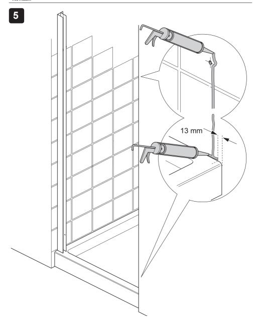
(a) Apply silicone sealant along the length of the wall and at the bottom where the wall channel will be placed.
