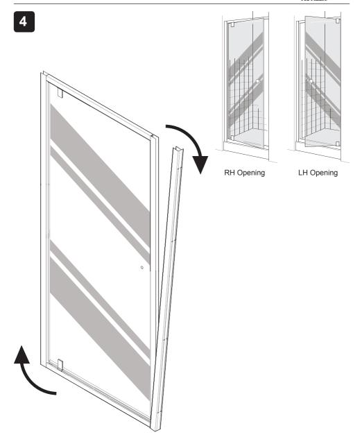
(a) The pivot door can be either a LH or a RH opening. To change the opening simply rotate the frame through 180° before continuing with the installation
