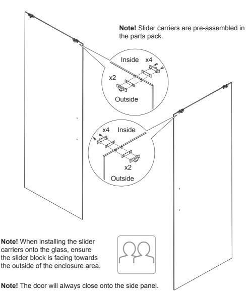
**Note!** To aid assembly, place the assembled door inside the enclosure prior to the fixed panels being installed.
