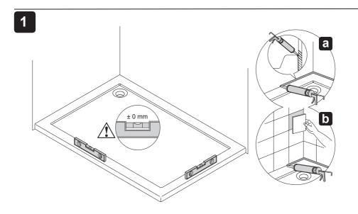
**Note!** Make sure that the walls have been tiled down to the tray. Make sure the tray is levelled. Make sure the walls are flat and square.
