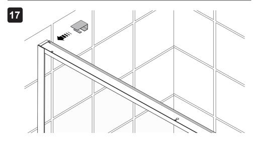
Select the correct handed bracket cover for your installation and push into place.
