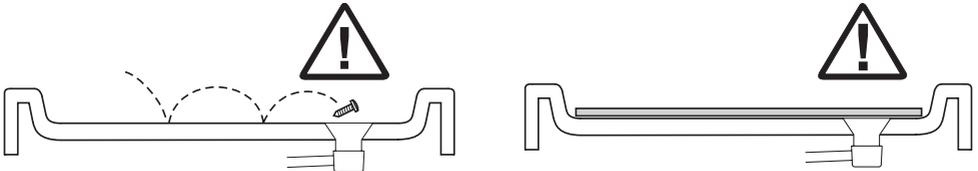
**Note!** Cover the tray waste to prevent the loss of small parts.
