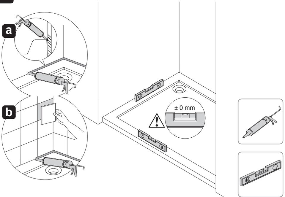
**Note!** Make sure that the walls have been tiled down to the tray. Make sure the tray is level. Make sure the walls are flat and square.
