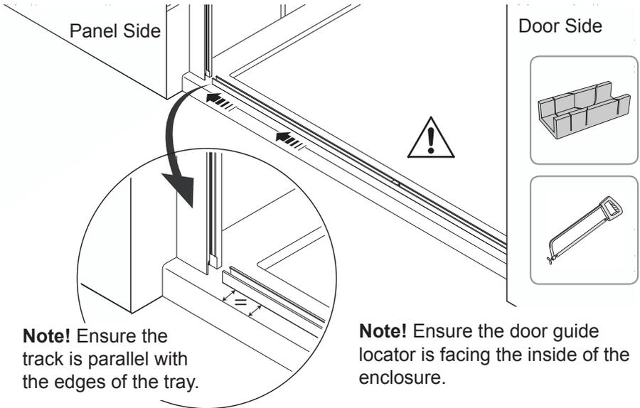
**Note!** Ensure the track is parallel with the edges of the tray.
