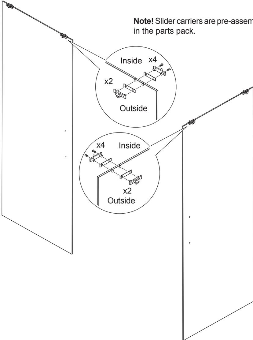
**Note!** To aid assembly, place the assembled door inside the enclosure prior to the fixed panel being installed.
