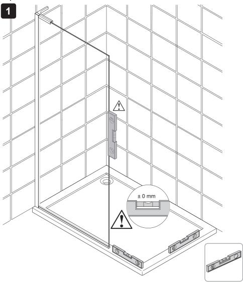
(a) Install the Divider Panel in accordance with the manufacturer's instructions. Caution! Make sure that the shower tray and divider panel are level.
